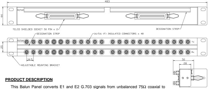
This Balun Panel converts E1 and E2 G.703 signals from unbalanced  $75\Omega$  coaxial to balanced  $120\Omega$  twisted pair transmissions. A bi-directional device requiring no external power, it allows the user to connect telecommunications equipment with mismatched interfaces. This product offers the following features:-
