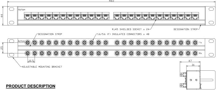
This Balun Panel converts E1 and E2 G.703 signals from unbalanced  $75\Omega$  coaxial to balanced  $120\Omega$  twisted pair transmissions. A bi-directional device requiring no external power, it allows the user to connect telecommunications equipment with mismatched interfaces or facilitates the conversion from coaxial to twisted pair distribution wiring. This product offers the following features:-
