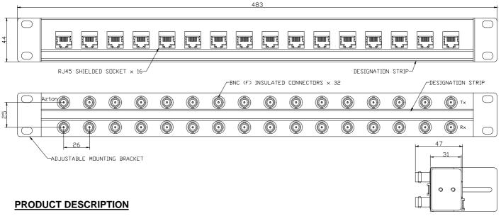
VIEW WITH BRACKET REMOVED This Balun Panel converts E1 and E2 G.703 signals from unbalanced 75 $\Omega$  coaxial to balanced 120Ω twisted pair transmissions. A bi-directional device requiring no external power, it allows the user to connect telecommunications equipment with mismatched interfaces or facilitates the conversion from coaxial to twisted pair distribution wiring. This product offers the following features:-
