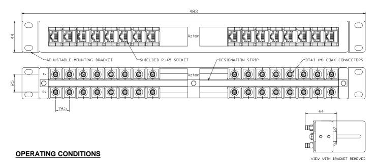
Matching Impedance: 75 ohm unbalanced coaxial to 120 ohm balanced twisted pair Bit Rate: 2Mbit/s (E1) and 8Mbit/s (E2) per ITU-T G.703 Line Code Signal Level: 2.37V nominal peak voltage at the coaxial end per G.703
