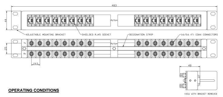
Matching Impedance: 75 ohm unbalanced coaxial to 120 ohm balanced twisted pair 2Mbit/s (E1) and 8Mbit/s (E2) per ITU-T G.703 Line Code Signal Level: 2.37V nominal peak voltage at the coaxial end per G.703
