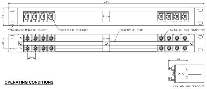
Matching Impedance: 75 ohm unbalanced coaxial to 120 ohm balanced twisted pair Bit Rate: 2Mbit/s (E1) and 8Mbit/s (E2) per ITU-T G.703 Line Code Signal Level: 2.37V nominal peak voltage at the coaxial end per G.703
